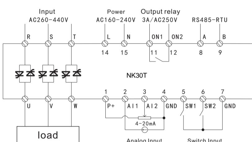
The default is stop start signal SW1, SW2 default switch between AI1 and AI2, closed AI2 given signal is valid, disconnect AI1 given signal is valid.
