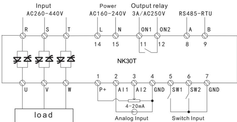
The default is stop start signal SW1, SW2 default switch between AI1 and AI2, closed AI2 given signal is valid, disconnect AI1 given signal is valid.
